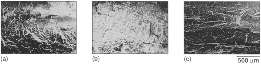
Fig. 3. Fracture surfaces of the blow-molded bottles of PE/MPAb samples pre-blended in a twin screw extruder before blow-molding with (a) 10%, (b) 20%, (c) 30% of MPAb.
